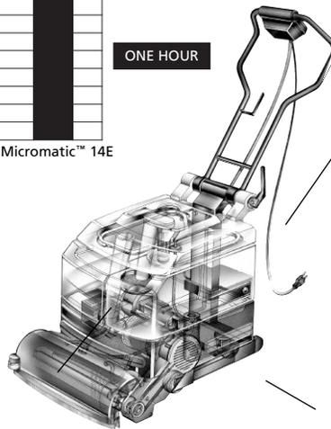
Simple, convenient controls for vacuum and brush on/off and min./max solution flow. A foot pedal raises, lowers and shifts the cleaning head, and is easy for even the inexperienced operator to master. The 14E is safe, quiet and comfortable to work with.
